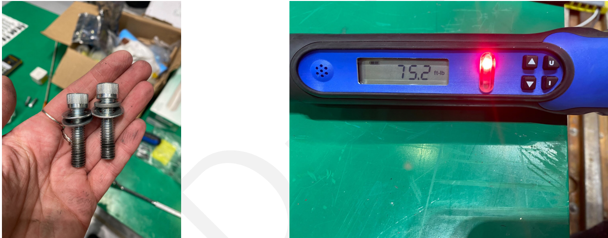
FIGURE 32: MEC-01. Two of the sheared 3/8-16 socket-head bolts recovered from the cable wrap, and the bolt test that followed a few days later: 75.2 ft-lb applied with no sign of failure (2025-01-30, #cam-summit-ops).
