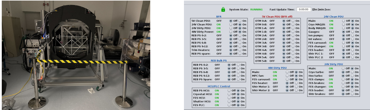
FIGURE 29: FES-03 . Left: an autochanger on its stand in the clean room, where the homing procedure was qualified (2025-04-07). Right: the quadbox power panel, whose FES carousel, clamp, loader and brake channels are the supplies behind the truck undervoltage faults (2025-02-13).
