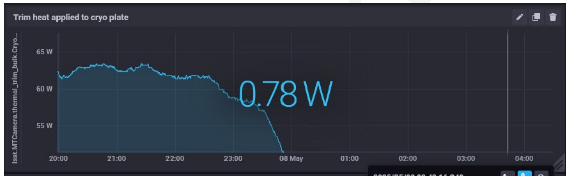
FIGURE 2: CRYO-01. Top: the 8 May loss of capacity as it was reconstructed afterwards — cryo temperatures, cryostat and heat-exchanger vacuum and the cryo-plate trim heat, with the moments the dome-closure decision was taken and completed marked (2025-05-27). Bottom: trim heat applied to the cryo plate falling to 0.78 W, the floor at which the plate can no longer be held in control (2025-05-25).
