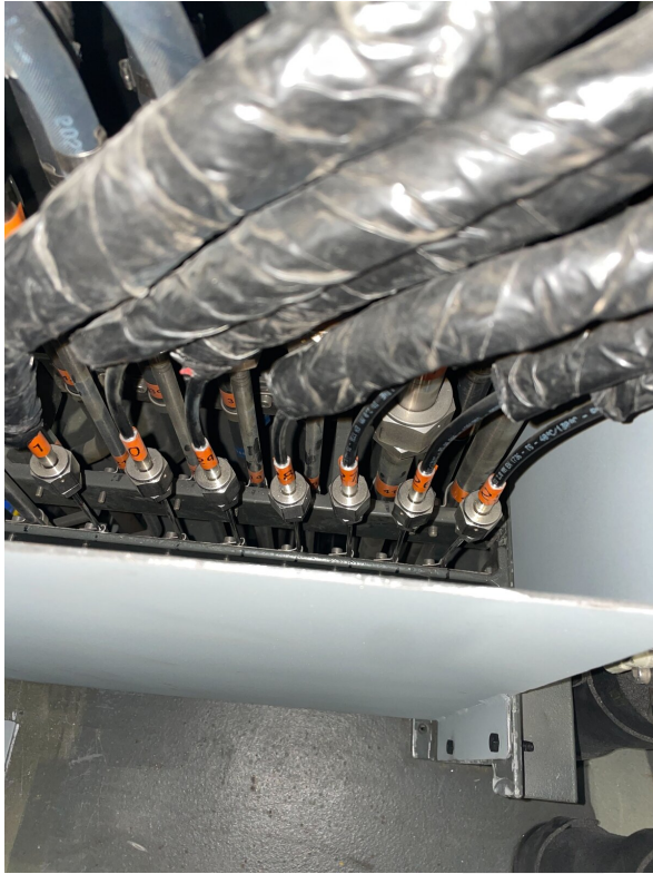
FIGURE 7: DYN-04. Refrigeration and Dynalene lines at the Top End Assembly, photographed during the June investigation of humidity and insulation in the camera region; the uninsulated runs of this kind are where the condensation found in December formed (2025-06-14).
