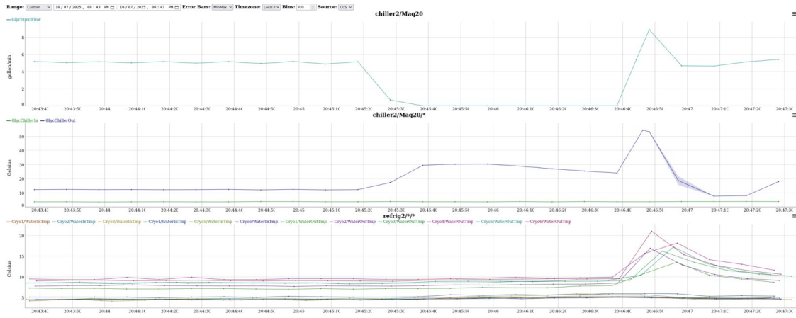
FIGURE 8: GLY-01 . One of the near misses, at second resolution. Glycol input flow to the PCS (top) drops from 5.2 gallons per minute to zero at 20:45:30 and is restored about 70 seconds later; the chiller outlet temperature (middle) had already climbed from 12 to 30°C before the interruption and overshoots to 54°C on restart, and the cryo water-out temperatures (bottom) follow it up. The chiller trips if the flow is lost for 90 to 120 seconds (2025-10-07, #cam-operator).
