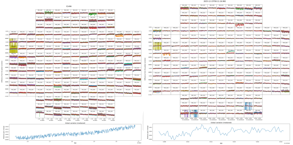
FIGURE 73: Difference of the per-amplifier relative gain from the focal-plane median, and the median itself (bottom panel of each plot). Left: without the natural frequency firmware (run E1496). Right: with the natural frequency firmware (2025-12-15).
