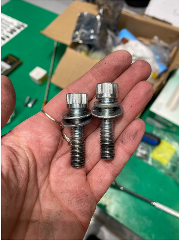
FIGURE 37: MEC-01. Two of the sheared 3/8-16 socket-head bolts recovered from the cable wrap, and the bolt test that followed a few days later: 75.2 ft-lb applied with no sign of failure (2025-01-30, #cam-summit-ops).
