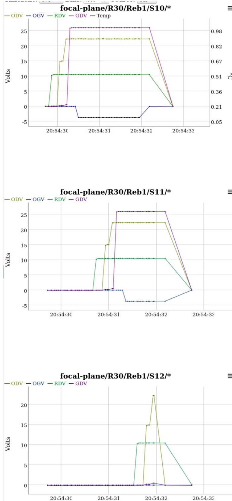
FIGURE 13: FP-01 . Bias voltages and currents on R30/Reb1 during the 7 April turn-on attempt, for S10, S11 and S12 from top to bottom; S10 and S11 follow the ramp while S12 trips off (2025-04-07, #cam-operator).
