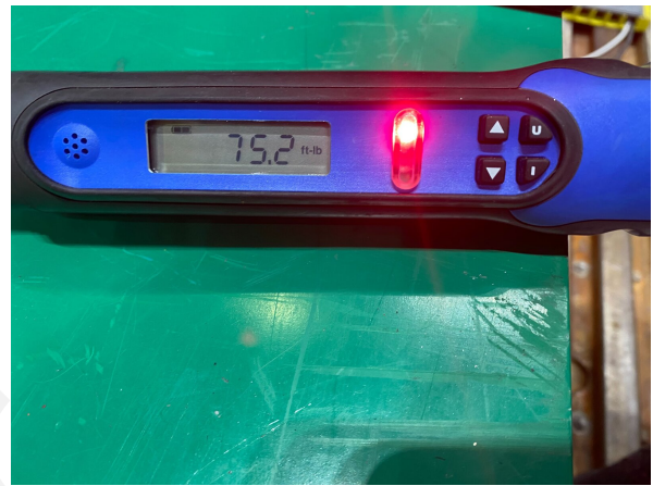
FIGURE 37: MEC-01. Two of the sheared 3/8-16 socket-head bolts recovered from the cable wrap, and the bolt test that followed a few days later: 75.2 ft-lb applied with no sign of failure (2025-01-30, #cam-summit-ops).
