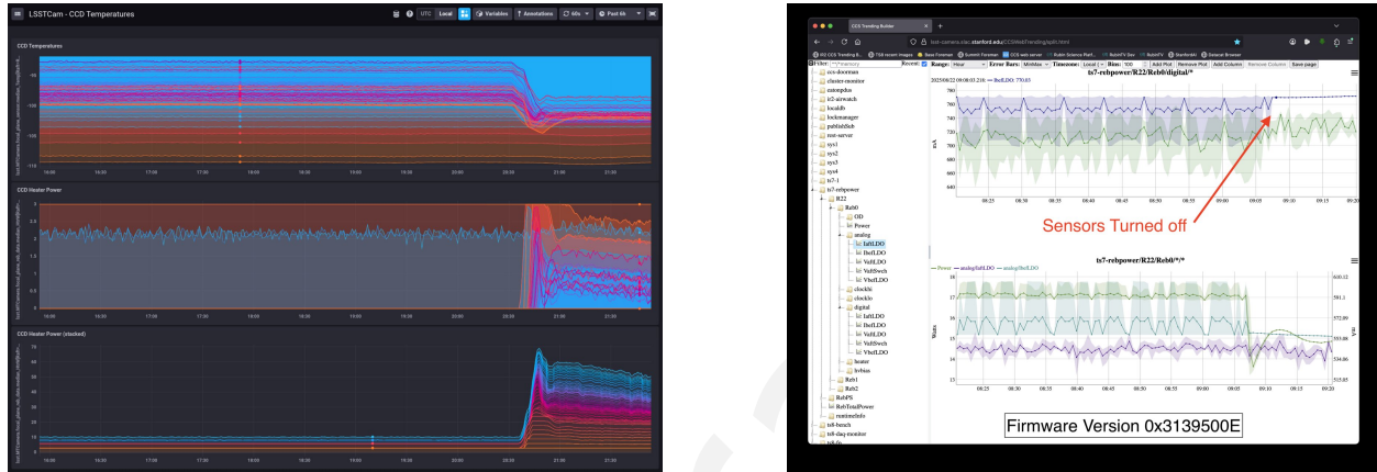
FIGURE 14: FW-01. Left: CCD temperatures and CCD heater power across the firmware roll-back, the step in heater power being the extra draw the faulty build was applying (2025-08-21). Right: the same measurement annotated during the investigation, with the moment the sensors were turned off marked and the firmware version under test named (2025-08-22).
