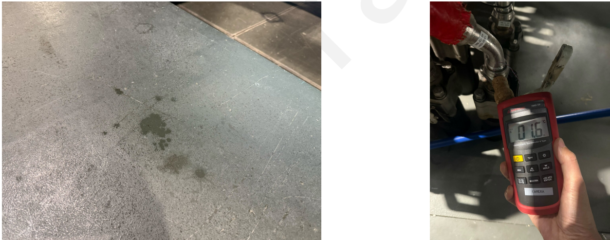
FIGURE 6: DYN-04. Left: the liquid found below the camera cable wrap on 16 December, a little left of centre looking into the mirror — the drops that were traced back to the Top End Assembly. Right: the source, measured a week later: an uninsulated Dynalene line at the cable wrap reading 1.6°C on its surface, well below the dew point of the air around it (2025-12-16 and 2025-12-24, #cam-summit-ops).
