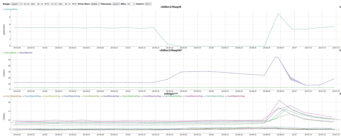
FIGURE 7: GLY-01 . One of the near misses, at second resolution. Glycol input flow to the PCS (top) drops from 5.2 gallons per minute to zero at 20:45:30 and is restored about 70 seconds later; the chiller outlet temperature (middle) had already climbed from 12 to 30°C before the interruption and overshoots to 54°C on restart, and the cryo water-out temperatures (bottom) follow it up. The chiller trips if the flow is lost for 90 to 120 seconds (2025-10-07, #cam-operator).
